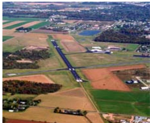
The crosswind runway (04/22) is 3,600 feet in length with a width of 100 feet and is constructed of bituminous concrete. Lighting aids on this runway include MIRLs and REILs on Runway 04. Instrument approaches to the airport include a Simplified Directional Facility to Runway 34, Non-directional Radio Beacon approach to Runway 04 and 16 and a Very High Frequency Omnidirectional Radio Range.
